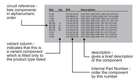
The mechanical and miscellaneous section lists the variant and common parts in IPN order.
